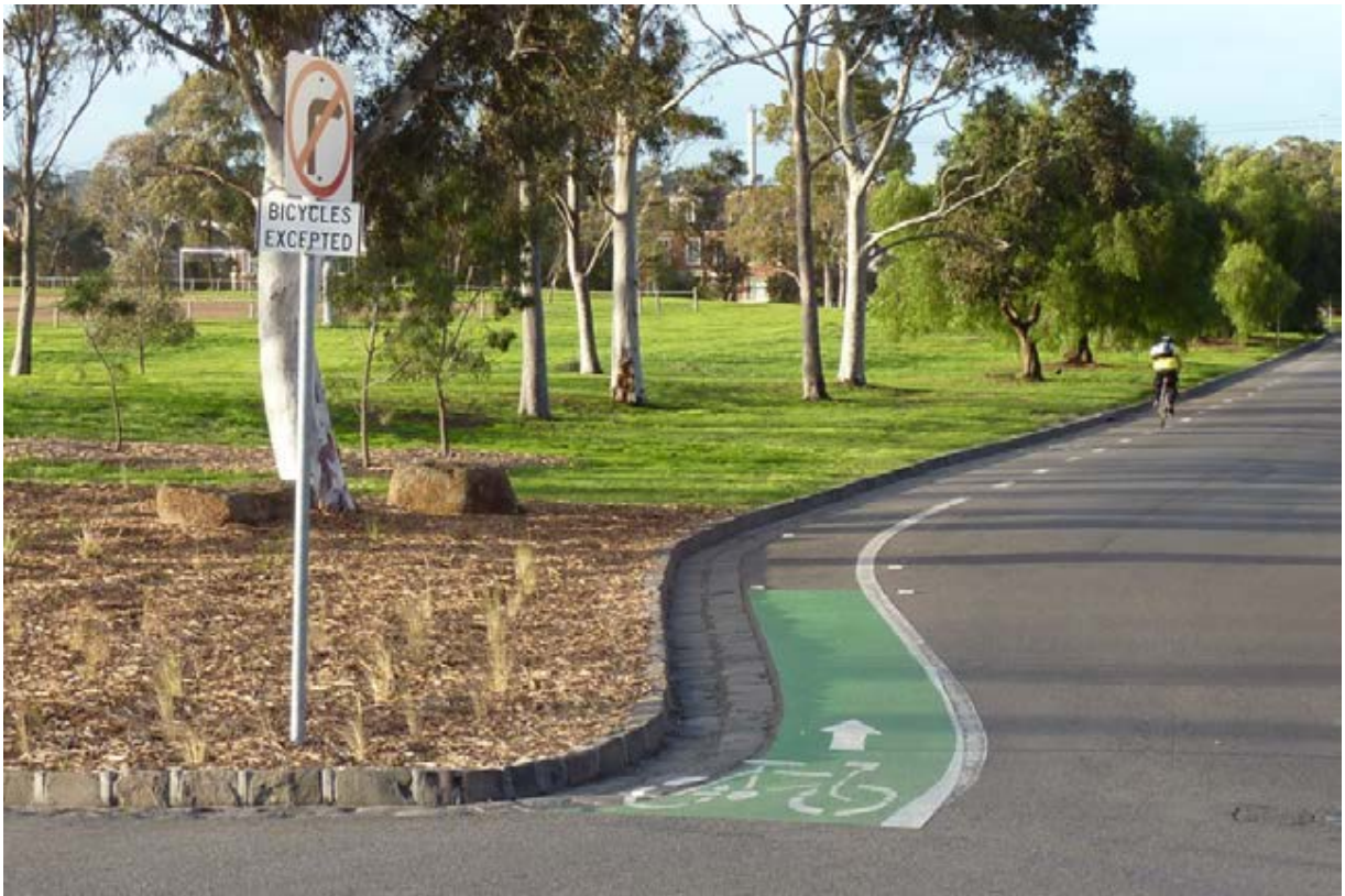
Figure 4.8: Contra-flow bicycle lane example
