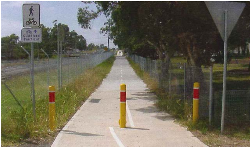
Figure 7.19: Example of a bollard treatment
