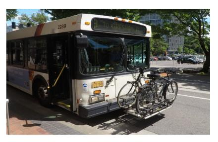
**Figure 8-5** TriMet bus in Portland with front-loading bicycle rack for two bicycles
