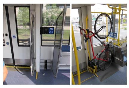
**Figure 8-7** Bicycle storage on light rail in Minneapolis and Portland, consisting of upright hanging cleats adjacent to door
