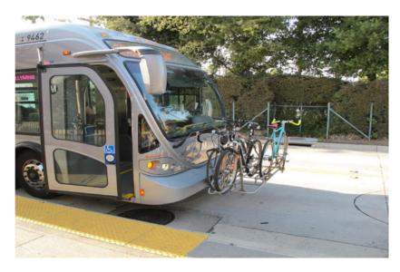
**Figure 8-6** Metro Orange Line BRT bus in Los Angeles with front-loading bicycle rack for three bicycles
