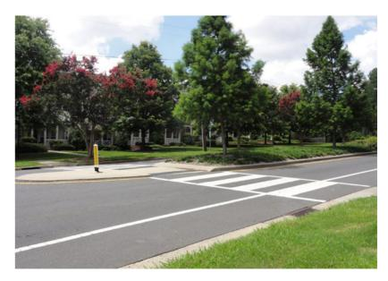
**Figure 5-4** Road diet on Clanton Road in Charlotte, NC (Photo: Rails-to-Trails Conservancy / trade.railstotrails.org)
